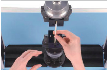
Operation with both hands by using the Foot Valve Unit
