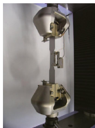
Fig. 2 Specimen and Jigs for Tensile Testing
